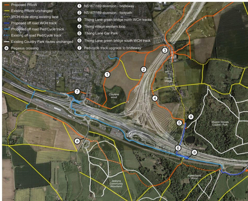
Plate A.7 Preliminary design: WCH routes in the M2/A2/A122 Lower Thames Crossing Junction area
